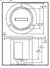
3 Screw Mount: Panel cutout 2.00 diameter opening Three .125 holes equally spaced on 2.42 bolt circle diameter\*
