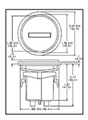
Flush Mount (Retainer) 2.24": Panel cutout 2.00 diameter opening\*
