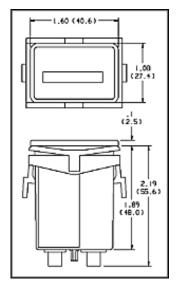
Retainer Mount: Panel cutout 1.45 x .95 rectangular opening. Two .150 holes spaced 1.750\*
