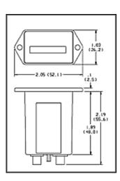
2 Screw Standard: Panel cutout 1.45 x .95 rectangular opening. Two .150 holes spaced 1.750\*
